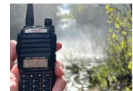
Figure 2: With the BTech GMRS-V2, you can quickly add or edit up to 200 GMRS or NOAA channels.
