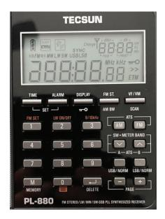
Pressing and holding the display/skeleton key button for 1 second locks or unlocks the keypad.
